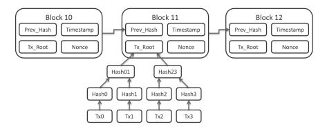
Figure 2: Blockchain, the underlying technology behind Bitcoin and all other cryptocurrencies, is simply a data structure consisting of an extended linked list of hash pointers with metadata. These pieces of metadata, in addition to carrying the actual BTC transaction information, more importantly serve data that can be used for efficient verification of double-spending in a distributed system [44].
