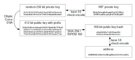
Figure 3: While public-key encryption is the basic idea behind the Bitcoin protocol, there are many additional details involved in making it a practical system to be used. In particular, additional hashing functions are used in an effort to make the underlying keys more manageable to deal with and store as an end user, while meeting sufficient security demands. These details, while interesting in their own right, however, are not of key important for this particular study [39].
