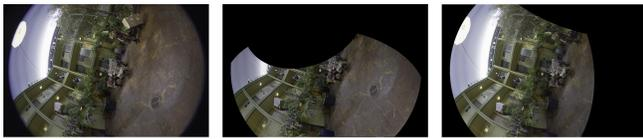
Fig. 10. Original color (left) and aligned projections of two overlapping cameras at infinity
